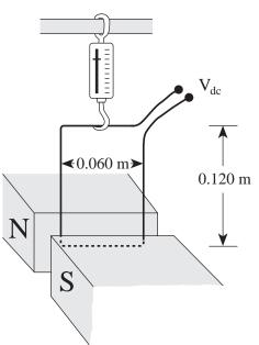
As the current in the loop is varied, the readings of the spring scale and current are plotted on a graph.
