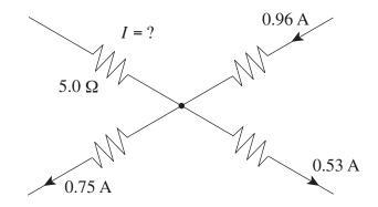
What is the current and its direction through the 5.0  $\Omega$  resistor?
